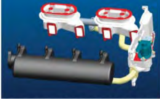
A schematic of the EGR system being used on Hatz's L and M Series diesel engines.
