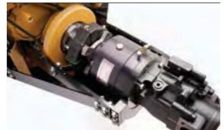
Logan PTO with 100 gpm pump. (Guards removed for clarity)
