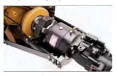
**Logan PTO with 100 gpm pump.** (Guards removed for clarity)
