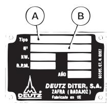
The model type A and the engine serial No. B are given in the engine identification rplate.
