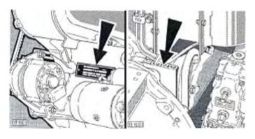
The engine identification plate is mounted to the crankcase.
