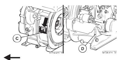
The engine identification plate C is located on the crankcase. The serial No. D is also stamped on the engine block.
