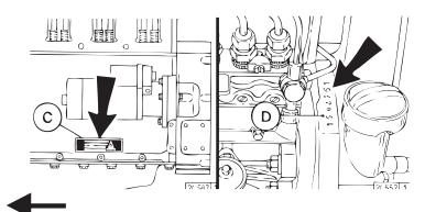
The engine identification plate C is mounted to the crankcase.
