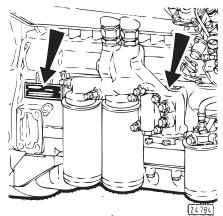
The engine identification plate is mounted to the crankcase at left of the lube filters and in the air cowling. The serial No. is also stamped into
