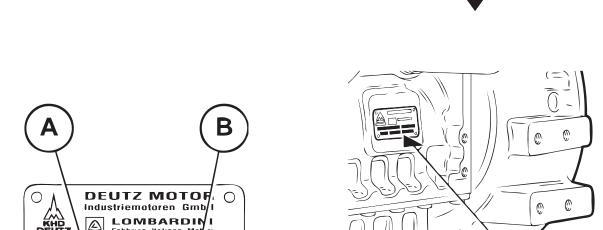
The model type A and the engine serial No. B are given in the engine identification plate.
