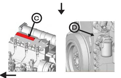
The engine identification plate C is mounted to the valve cover.
