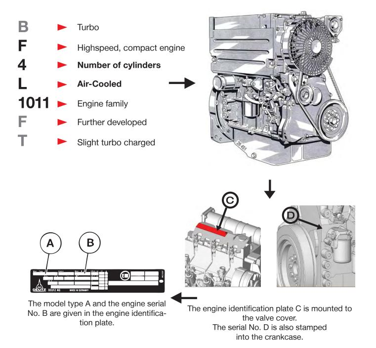
For integrated cooled engines with air discharge duct the engine identification plate is located between cooling blower housing and air duct.
