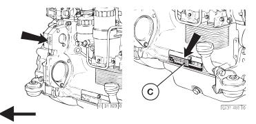
The engine identification plate C is mounted to the crankcase. The serial No. is also stamped into the crankcase.
