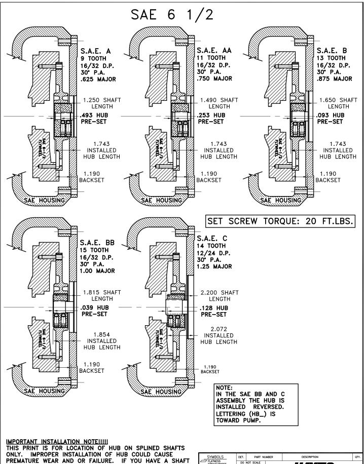
THIS PRINT IS FOR LOCATION OF HUB ON SPLINED SHAFTS ONLY. IMPROPER INSTALLATION OF HUB COULD CAUSE PREMATURE WEAR AND OR FAILURE. IF YOU HAVE A SHAFT LENGTH OTHER THAN THOSE SHOWN HERE PLEASE CONTACT DISTRIBUTOR OR FACTORY FOR FURTHER INFORMATION. HUB SET SCREWS MUST BE PROPERLY TORQUED TO 20 FT.LBS. EACH. PLEASE CONTACT DISTRIBUTOR OR FACTORY FOR ANY FURTHER QUESTIONS.
