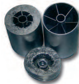
Sectioned rotor full with contaminant. Sectioned rotor displaying the internal ribs.
